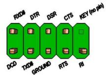
Figure 8 Serial port header pin-out
