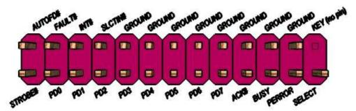
Figure 7 Parallel port header pin-out
