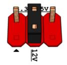
Pins 3&4: jumper position for 12V
